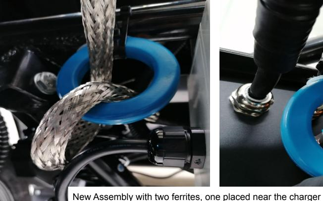
and the other near the battery. Fix the ferrites with plastic clamps as shown in the pictures..
